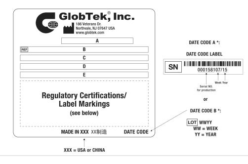
A=ICT / ITE / Medical Power Supply/Class 2/Household Power Supply B=P/N: (料号) WR9QA3000USBC-CIMR6W C=Model (型号) GTM96180-1507-2.0 D=Input (输入)100-240V~, 50-60 Hz, 0.6 A E=Output (输出)5.0 V ---- 3.0 A, 15.00W
