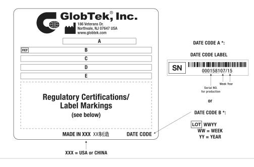
A=ICT / ITE / Medical Power Supply/Class 2/Household Power Supply B=P/N: (料号) WR9QA3000MICBCMR6B C=Model (型号) GTM96180-1607-1.8 D=Input (输入)100-240V~, 50-60 Hz, 0.6 A E=Output (输出)5.2 V ---- 3.07 A, 16.00W
