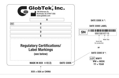
A=ICT / ITE / Medical Power Supply/Class 2/Household Power Supply B=P/N: (料号) WR9QA3000LLPCIMR6B C=Model (型号) GTM96180-1507-2.0 D=Input (输入)100-240V~, 50-60 Hz, 0.6 A E=Output (输出)5.0 V ---- 3.0 A, 15.00W
