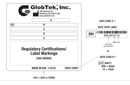
A=ICT / ITE / Medical Power Supply/Class 2/Household Power Supply B=P/N: (料号) WR9QA1500USBCNACIMR6B C=Model (型号) GTM96180-0807-2.0 D=Input (输入)100-240V~, 50-60 Hz, 0.6 A E=Output (输出)5.0 V ---- 1.5 A, 7.50W
