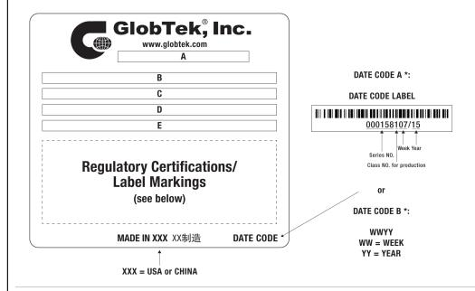
A=ICT / ITE / Medical Power Supply/Class 2/Household Power Supply B=P/N: (料号) WR9QA1200T00NAIMR6B C=Model (型号) GTM96060-0606-1.0 D=Input (输入)100-240V~, 50-60 Hz, 0.6 A E=Output (输出)5.0 V == 1.2 A, 6.00W
