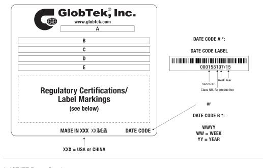
A=ICT/ITE Power Supply B=P/N: (料号) WR9QA1200MICB-N(R6B) C=Model (型号) GT-46060-0605 D=Input (输入)100-240V~, 50-60 Hz, 0.3 A E=Output (输出)5.0 V ---- 1.2 A, 6.00W
