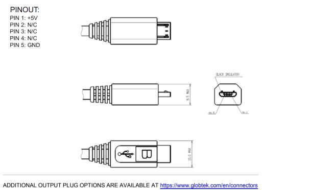
STANDARD PLUGS AND CONNECTORS CAN BE SEEN ONLINE AT https://www.globtek.com/en/connectors CALCULATE VOLTAGE REGULATION/DROP WITH OUR ONLINE CALCULATOR: https://www.globtek.com/r2/PtqjjL
