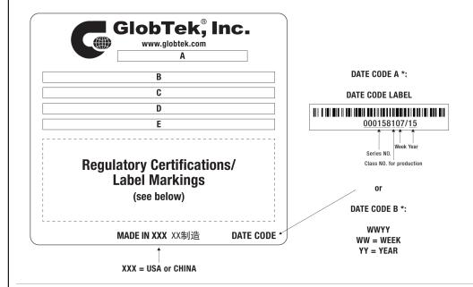
A=ICT / ITE / Medical Power Supply/Class 2/Household Power Supply B=P/N: (料号) WR9QA1200MAG2C2A-R6B C=Model (型号) GTM96060-0606-1.0 D=Input (输入)100-240V~, 50-60 Hz, 0.6 A E=Output (输出)5.0 V == 1.2 A, 6.00W
