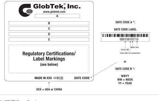
A=ICT/ITE Power Supply B=P/N: (料号) WR9ME500LCP-F(R6B) C=Model (型号) GT-86060-0612-W2E D=Input (输入)100-240V~, 50/60Hz, 0.2A E=Output (输出)12.0 V === 0.5 A, 6.00W
