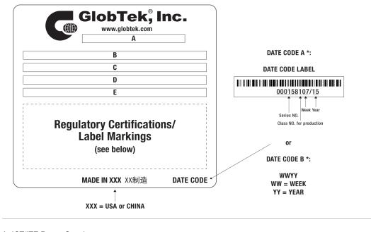
A=ICT/ITE Power Supply B=P/N: (料号) WR9ME3000CCP-F(R6B) C=Model (型号) GT-83082-3612-W2E D=Input (输入)100-240V~, 50-60 Hz, 1.0A E=Output (输出)12.0 V == 3.0 A, 36.00W
