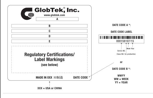
A=ICT/ITE Power Supply B=P/N: (料号) WR9ME2000CCP-F(R6B) C=Model (型号) GT-86240-2412-W2E D=Input (输入)100-240V~, 50-60Hz, 1A E=Output (输出)12.0 V == 2.0 A, 24.00W
