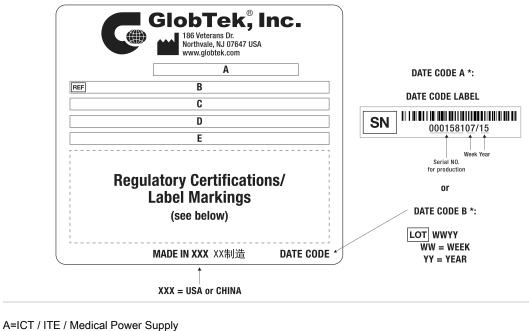
A=IC1 / ITE / Medical Power Supply B=P/N: (料号) WR9ME1000LCPIMFR6B C=Model (型号) GTM86101-1212-W2E D=Input (输入)100-240V~, 50-60Hz, 0.3A E=Output (输出)12.0 V --- 1.0 A, 12.00W
