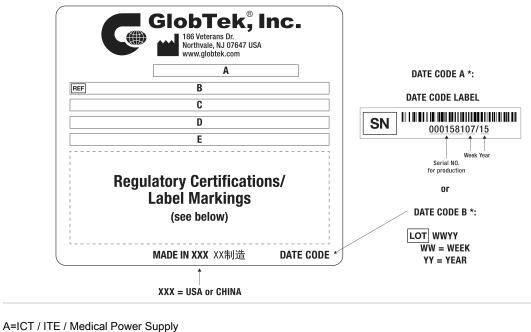
B=P/N: (料号) WR9MD1110LCPIMFR6B C=Model (型号) GTM86101-1009-W2E D=Input (输入)100-240V~, 50-60Hz, 0.3A E=Output (输出)9.0 V === 1.11 A, 10.00W
