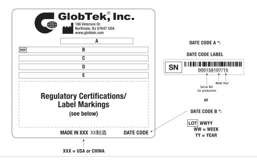
A=ICT / ITE / Medical Power Supply B=P/N: (料号) WR9MD1110CCPIMFR6B C=Model (型号) GTM86101-1009-W2E D=Input (输入)100-240V~, 50-60Hz, 0.3A E=Output (输出)9.0 V === 1.11 A, 10.00W
