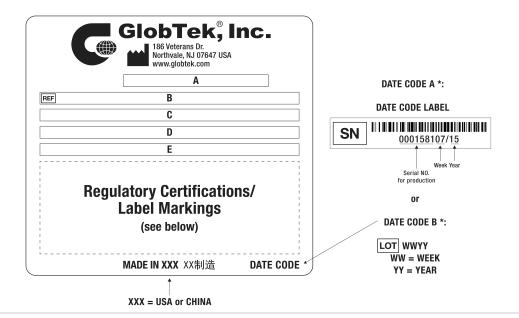
A=ICT / ITE / Medical Power Supply B=P/N: (料号) WR9MB2000LCPIMFR6B C=Model (型号) GTM86101-1205.95-W2E D=Input (输入)100-240V~, 50-60Hz, 0.3A E=Output (输出)5.95 V == 2.01 A, 12.00W
