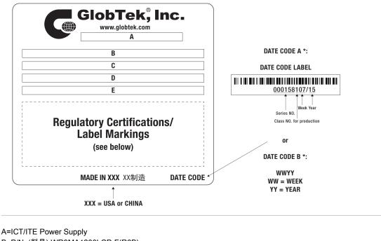
B=P/N: (料号) WR9MA1200LCP-F(R6B) C=Model (型号) GT-86060-0505-W2E D=Input (输入)100-240V~, 50/60Hz, 0.2A E=Output (输出)5.0 V == 1.2 A, 6.00W
