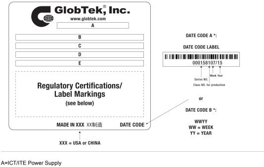
B=P/N: (料号) WR9MA1000USB-F(R6B) C=Model (型号) GT-83083-0505-USB-W2E D=Input (输入)100-240¼, 50/60Hz, 0.2A E=Output (输出)5.0 V ---- 1.0 A, 5.00W
