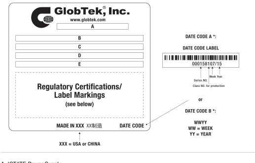
A=ICT/ITE Power Supply B=P/N: (料号) WR9HU1800CCP-F(R6B) C=Model (型号) GT-86181-1810 -W2 D=Input (输入)100-240V-, 50/60Hz, 0.6 A E=Output (输出)10.0 V === 1.8 A, 18.00W
