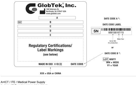
B=P/N: (料号) WR9HI500LCPIMFR6B C=Model (型号) GTM86101-1224-W2 D=Input (输入)100-240V~, 50-60Hz, 0.5A E=Output (输出)24.0 V --- 0.5 A, 12.00W
