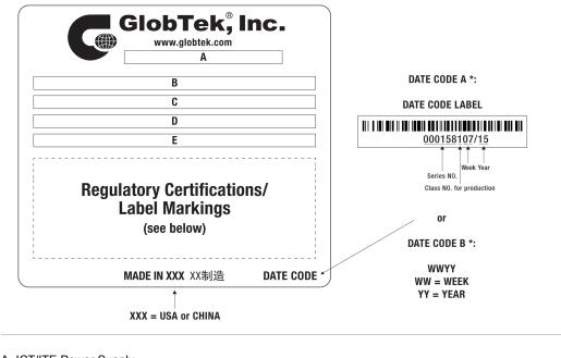
A=ICT/ITE Power Supply B=P/N: (料号) WR9HG1200LCP-F(R6B) C=Model (型号) GT-86181-1815 -W2 D=Input (输入)100-240V-, 50/60Hz, 0.6 A E=Output (输出)15.0 V == 1.2 A, 18.00W
