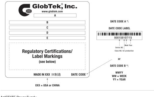
A=ICT/ITE Power Supply B=P/N: (料号) WR9HE500CCP-F(R6B) C=Model (型号) GT-86060-0612-W2 D=Input (输入)100-240V-, 50/60Hz, 0.2A E=Output (输出)12.0 V == 0.5 A, 6.00W
