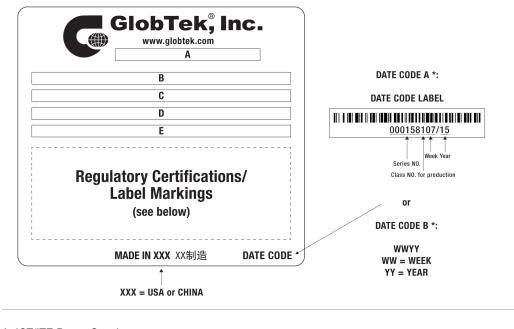
A=ICT/ITE Power Supply B=P/N: (料号) WR9HE2000C9P-F(R6B) C=Model (型号) GT-86240-2412-W2 D=Input (输入)100-240V~, 50-60Hz, 0.8A E=Output (输出)12.0 V == 2.0 A, 24.00W
