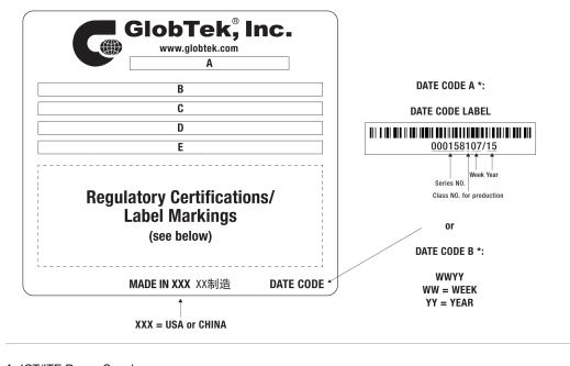
A=ICT/ITE Power Supply B=P/N: (料号) WR9HE1000LLP-F(R6B) C=Model (型号) GT-86120-1212-W2 D=Input (输入)100-240V-, 50/60Hz, 0.5A E=Output (输出)12.0 V == 1.0 A, 12.00W
