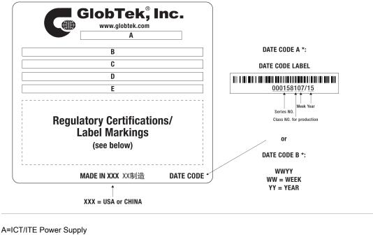
B=P/N: (料号) WR9HD2000LCP-F(R6B) C=Model (型号) GT-86181-1809 -W2 D=Input (输入)100-240V-, 50/60Hz, 0.6 A E=Output (输出)9.0 V == 2.0 A, 18.00W
