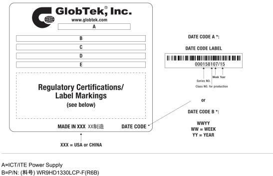
C=Model (型号) GT-86121-1209-W2 D=Input (输入)100-240V-, 50/60Hz, 0.5A E=Output (输出)9.0 V --- 1.33 A, 12.00W
