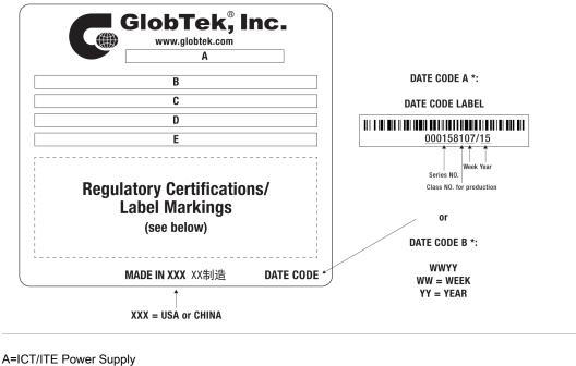
B=P/N: (料号) WR9HB1680LCP-F(R6B) C=Model (型号) GT-86120-1012-6.05-W2 D=Input (输入)100-240V-, 50/60Hz, 0.5A E=Output (输出)5.95 V === 1.68 A, 10.00W
