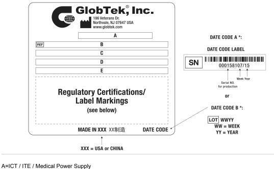
B=P/N: (料号) WR9HA2000USBFMR6B C=Model (型号) GTM86100-1005-W2-USB D=Input (输入)100-240V~, 50-60 Hz, 0.3A E=Output (输出)5.0 V == 2.0 A, 10.00W
