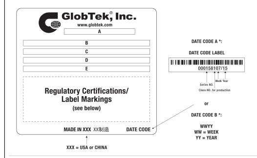
A=ICT / ITE / Medical Power Supply B=P/N: (料号) WR9HA2000MICB-MFR6B C=Model (型号) GTM86100-1005-W2 D=Input (输入)100-240V~, 50-60Hz, 0.3A E=Output (输出)5.0 V == 2.0 A, 10.00W
