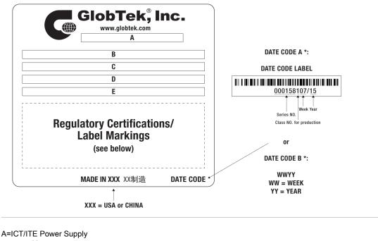
B=P/N: (料号) WR9HA2000LCP-F(R6B) C=Model (型号) GT-86120-1005-W2 D=Input (输入)100-240V-, 50/60Hz, 0.5A E=Output (输出)5.0 V == 2.0 A, 10.00W
