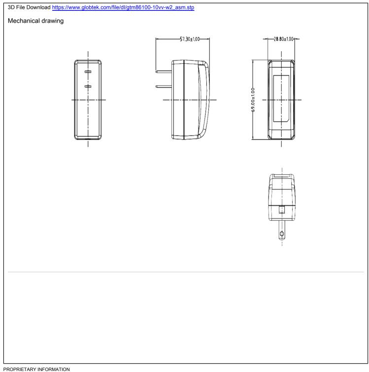
PROPRIETARY INFORMATION PROPRIETARY OF GLOBTEK, INC. ANY REPRODUCTION, DISCLOSURE OR USE OF THIS DRAWING, IN WHOLE OR IN PART, IS HEREBY PROHIBITED EXCEPT AS SPECIFIED IN WRITING BY GLOBTEK, INC. © GlobTek, Inc. 2022 - 2025 guest / 05/20/2025 6:15:16 AM GMT CLONED FROM WR9HA2000CCPMFR6B
