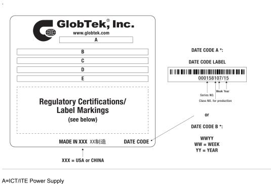
B=P/N: (料号) WR97E1000L14PFR6B C=Model (型号) GT-86120-1212-W2A D=Input (输入)100-240V-, 50/60Hz, 0.5A E=Output (输出)12.0 V == 1.0 A, 12.00W
