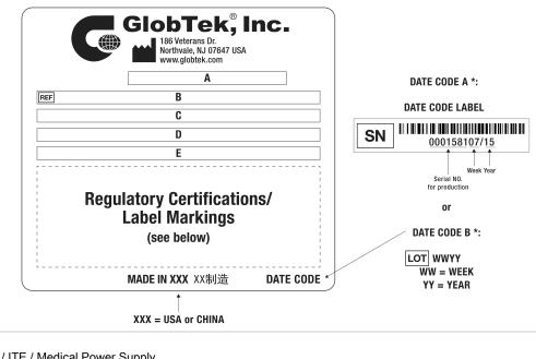
A=ICT / ITE / Medical Power Supply B=P/N: (料号) WR97A2000MICB-MFR6B C=Model (型号) GTM86100-1005-W2A D=Input (输入)100-240V~, 50-60Hz, 0.3A E=Output (输出)5.0 V --- 2.0 A, 10.00W
