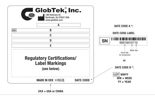
A=ICT / ITE / Medical Power Supply B=P/N: (料号) WR95I500LCPIMFR6B C=Model (型号) GTM86101-1224-W2U D=Input (输入)100-240V~, 50-60Hz, 0.3A E=Output (输出)24.0 V == 0.5 A, 12.00W
