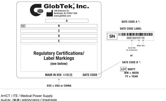
B=P/N: (料号) WR95G800LCPIMFR6B C=Model (型号) GTM86101-1215-W2U D=Input (输入)100-240V~, 50-60Hz, 0.3A E=Output (输出)15.0 V --- 0.8 A, 12.00W
