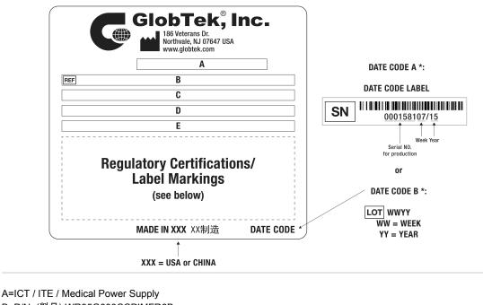
B=P/N: (料号) WR95G800CCPIMFR6B C=Model (型号) GTM86101-1215-W2U D=Input (输入)100-240V~, 50-60Hz, 0.3A E=Output (输出)15.0 V --- 0.8 A, 12.00W
