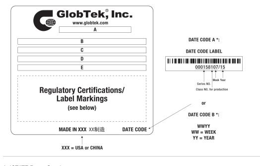
A=ICT/ITE Power Supply B=P/N: (料号) WR95E1500LCP-F(R6B) C=Model (型号) GT-86180-1812-W2U D=Input (输入)100-240V~, 50-60 Hz, 0.6 A E=Output (输出)12.0 V === 1.5 A, 18.00W
