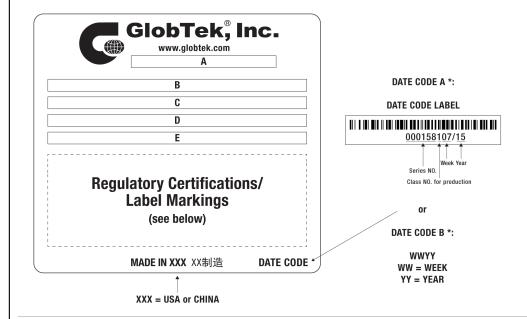
A=ICT / ITE / Medical Power Supply/Class 2/Household Power Supply B=P/N: (料号) TR9WZ3157T00CIMR6B C=Model (型号) GTM96600-6019-T2A D=Input (输入)100-240V~, 50-60Hz, 1.5A E=Output (输出)19.0 V === 3.16 A, 60.00W
