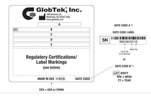
A=ICT / ITE / Medical Power Supply/Class 2/Household Power Supply B=P/N: (料号) TR9WX1250T00CIMR6B C=Model (型号) GTM96600-6048-T2A D=Input (输入)100-240V~, 50-60Hz, 1.5A E=Output (输出)48.0 V == 1.25 A, 60.00W
