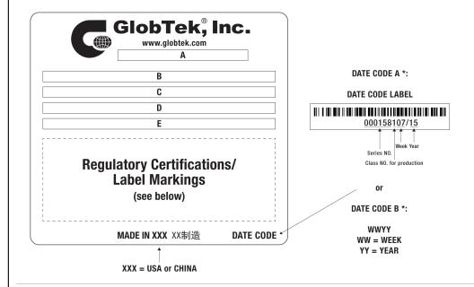
A=ICT / ITE / Medical Power Supply/Class 2/Household Power Supply B=P/N: (料号) TR9WR2000T00CIMR6B C=Model (型号) GTM96600-6030-T2A D=Input (输入)100-240V~, 50-60Hz, 1.5A E=Output (输出)30.0 V == 2.0 A, 60.00W
