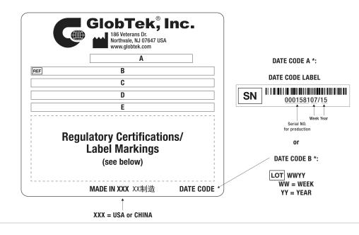
A=ICT / ITE / Medical Power Supply/Class 2/Household Power Supply B=P/N: (料号) TR9WI2500CCPCIMR6B C=Model (型号) GTM96600-6024-T2A D=Input (输入)100-240V~, 50-60Hz, 1.5A E=Output (输出)24.0 V === 2.5 A, 60.00W
