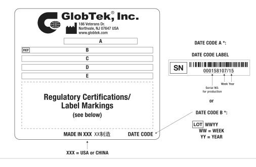
A=ICT / ITE / Medical Power Supply/Class 2/Household Power Supply B=P/N: (料号) TR9WG4000T00CIMR6B C=Model (型号) GTM96600-6015-T2A D=Input (输入)100-240V~, 50-60Hz, 1.5A E=Output (输出)15.0 V === 4.0 A, 60.00W
