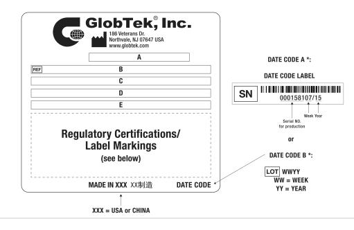
A=ICT / ITE / Medical Power Supply/Class 2/Household Power Supply B=P/N: (料号) TR9WA8000LCPIM(R6B) C=Model (型号) GTM96600-4005-T2A D=Input (输入)100-240V~, 50-60Hz, 1.5A E=Output (输出)5.0 V === 8.0 A, 40.00W
