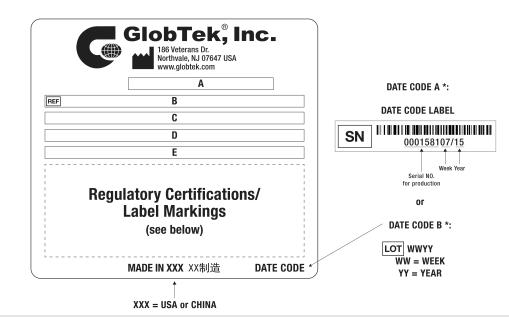
A=ICT / ITE / Medical Power Supply/Class 2/Household Power Supply B=P/N: (料号) TR9WA8000CCPIM(R6B) C=Model (型号) GTM96600-4005-T2A D=Input (输入)100-240V~, 50-60Hz, 1.5A E=Output (输出)5.0 V === 8.0 A, 40.00W
