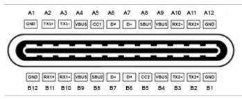
A1, A12, B1, B12: GND A4, A9, B4, B9: V+ CC1: A5 CC2: B5 D+: A6, B6 D-: A7, B7
