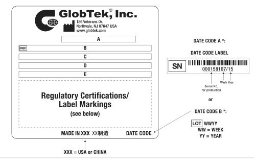
A=Medical/ICT/ITE/Household use Power Supply B=P/N: (料号) TR9KZ8421LCPIMR6B C=Model (型号) GTM961600P16019-T2 D=Input (输入)100-240V~, 50-60 Hz, 2.2A E=Output (输出)19.0 V === 8.42 A, 160.00W
