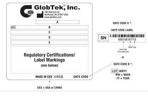
A=Medical/ICT/ITE/Household use Power Supply B=P/N: (料号) TR9KZ8421CCPIMR6B C=Model (型号) GTM961600P16019-T2 D=Input (输入)100-240V~, 50-60 Hz, 2.2A E=Output (输出)19.0 V === 8.42 A, 160.00W
