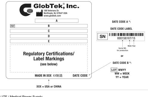
A=ICT / ITE / Medical Power Supply B=P/N: (料号) TR9KZ6316T00-IM(R6B) C=Model (型号) GTM961200P12019-T2 D=Input (输入)100-240V~, 50-60 Hz, 1.5 A E=Output (输出)19.0 V == 6.31 A, 120.00W
