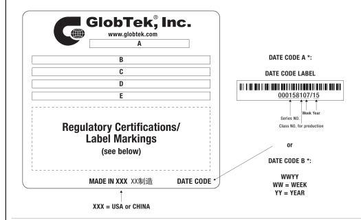
A=ICT / ITE / Medical Power Supply/Class 2/Household Power Supply B=P/N: (料号) TR9KZ3160LCPCIMR6B C=Model (型号) GTM96600-6019-T2 D=Input (输入)100-240V~, 50-60Hz, 1.5A E=Output (输出)19.0 V === 3.16 A, 60.00W
