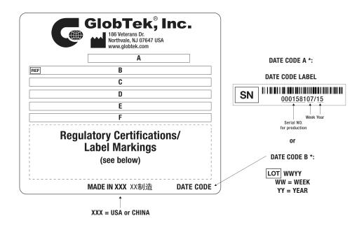
A=USB Power Delivery (PD) Source, ICT/ITE/Medical B=P/N: (料号) TR9KZ3000USBCFG2R6B C=Model (型号) GTM96605-G2A1-T2 D=Input (输入)100-240V~, 50-60Hz, 1.5A
