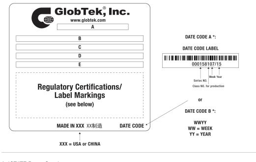
A=ICT/ITE Power Supply B=P/N: (料号) TR9KZ2105LCP-N(R6B) C=Model (型号) GT-46400-4019-T2 D=Input (输入)100-240V~, 50-60 Hz, 1.0A E=Output (输出)19.0 V == 2.1 A, 40.00W
