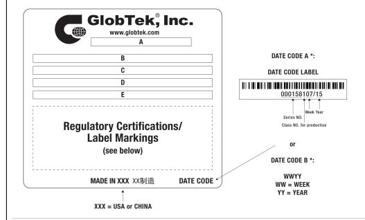
A=ICT / ITE / Medical Power Supply/Class 2/Household Power Supply B=P/N: (料号) TR9KX1350T00CIMR6B C=Model (型号) GTM96600-6548-T2 D=Input (输入)100-240V~, 50-60Hz, 1.5A E=Output (输出)48.0 V === 1.35 A, 65.00W
